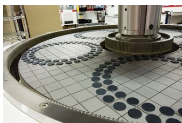
Click to Enlarge ND Filters Being Manufactured in Our Optics Production Facility
